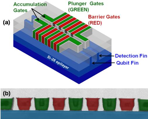
**Fig 1:** (a): Schematic of a quantum dot device showing multiple plunger, barrier, and accumulation gates, with active qubit and detection fins. (b) Cross-sectional TEM image through a qubit fin showing the various gates used to define the electrostatic landscape in the device and confine/couple individual electrons.
