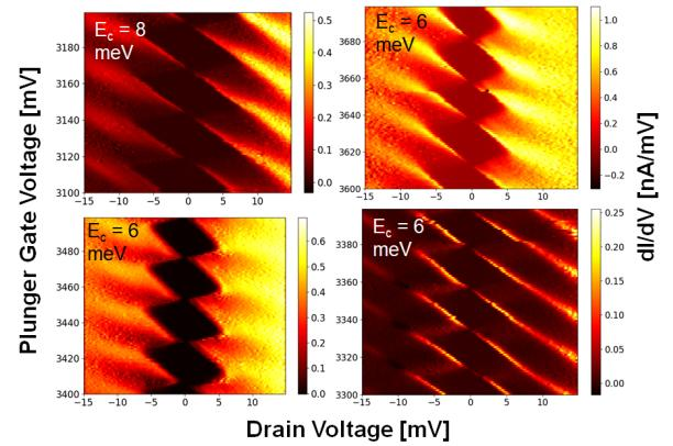
**Fig 13:** Corresponding Coulomb diamond data, measured at  $10\text{ mK}$ , to the blockade data shown in Fig 12. The differential conductance is plotted against drain voltage (x-axis) and plunger gate voltage (y-axis). The data show reproducible charging energies in the range of  $6\text{-}8\text{ mV}$ .
