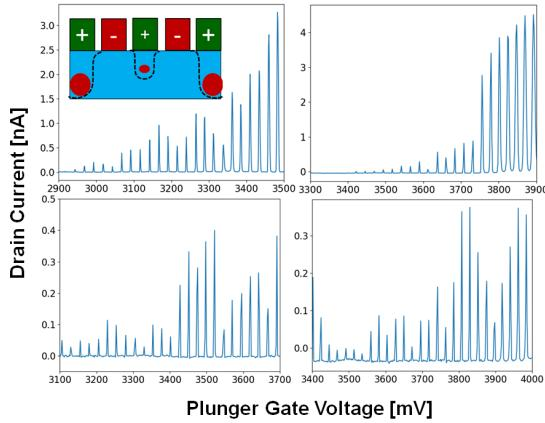
**Fig 12:** Coulomb blockade data measured at  $T = 10\text{ mK}$ . Each panel corresponds to data measured from different gates on different devices and indicate high quality reproducible dot formation. Inset: In the measurement the plunger gate (middle) is swept, while the adjacent gates are used to create a barrier potential. Other gates are biased to sufficient  $V_G - V_T$  to induce significant electron density.
