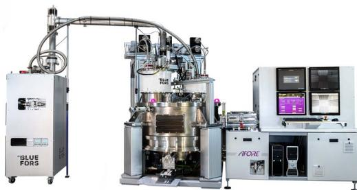
**Fig 4:** Prototype Cryogenic Wafer Prober. The tool allows full 300mm e-test automation at a wafer temperature of T= 1.9K.
