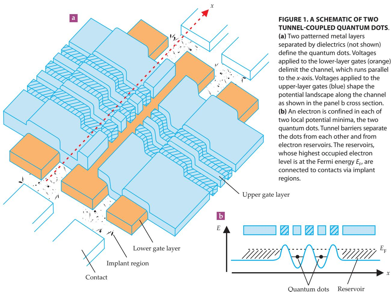
**FIGURE 1. A SCHEMATIC OF TWO TUNNEL-COUPLED QUANTUM DOTS.**
