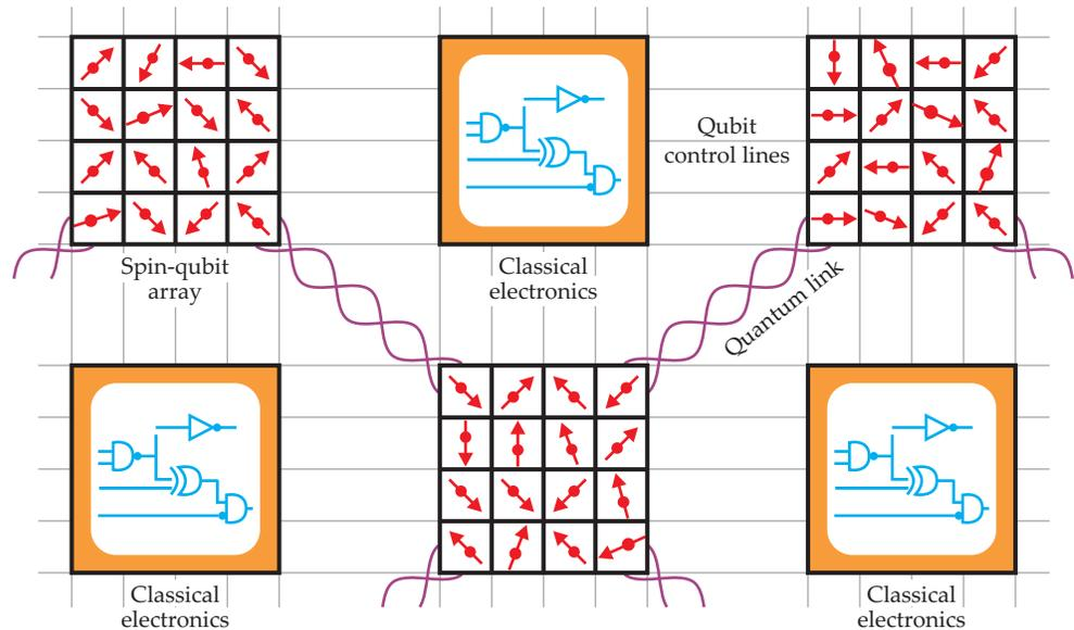
**FIGURE 5. A VISION OF FUTURE SILICON QUANTUM ELECTRONICS,** containing dense local registers of quantum dots interconnected with quantum links. Classical electronics between the spin-qubit arrays distribute signals on the chip.
