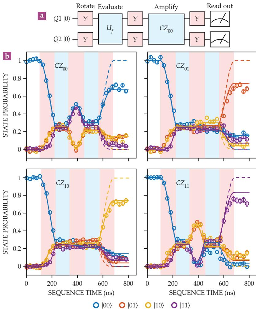
**FIGURE 4. A TWO-QUBIT CIRCUIT THAT IMPLEMENTS A QUANTUM SEARCH ALGORITHM.**
