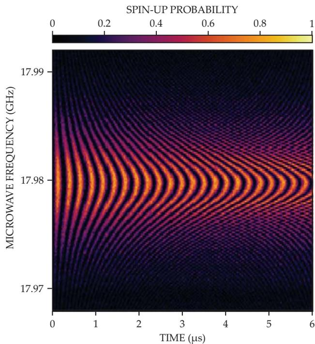
**FIGURE 2. DRIVEN EVOLUTION OF A SINGLE QUBIT.** When an applied microwave pulse is close to resonance with the spin qubit—that is, with the energy difference between its up and down states (17.98 GHz here)—the qubit undergoes driven rotations, or Rabi oscillation, and the probability of finding it spin-up oscillates as a function of the pulse duration. (Adapted from ref. 10.)
