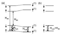
FIG. 20. Two views on spin relaxation due to the spin-orbit interaction and the phonon bath. (a) The electron phonon interaction does not couple pure spin states, but it does couple the spin-orbit perturbed spin states, labeled with superscripts <sup>(1)</sup>. Here  $\mathcal{H}_{SO}$  and  $\mathcal{H}_{e,\mathrm{ph}}$  are treated sequentially (although they do not commute). (b) The combined electron-phonon and spin-orbit Hamiltonian couples pure spin states.
