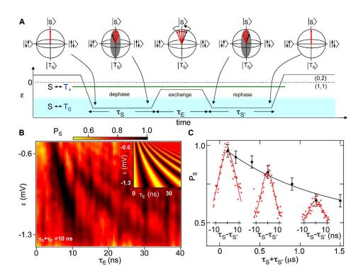
FIG. 49. (Color online) Error correction. (a) Singlet-triplet spin-echo pulse sequence. (b) Singlet state probability  $P_S$  measured as a function of pulse time  $\tau_E$  and detuning  $\varepsilon$ . Clear singlet state recoveries are observed for  $\pi$ ,  $3\pi$ ,  $5\pi$  exchange pulses. (c) The singlet state recovery persists out to  $T_2$  = 1.2  $\mu$ s. Data reproduced from Petta, Johnson, Taylor, *et al.*, 2005.
