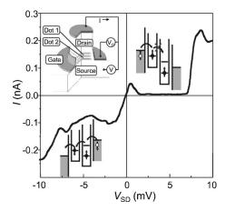
FIG. 33. Current (I) measured as a function of source-drain voltage (V) in a vertical double dot system. Nonzero current is measured over the entire range of negative voltage. For positive bias, current is blocked in the range 2 < V < 7 mV. At bias voltages exceeding 7 mV, the (0,2) triplet state becomes accessible and Pauli blockade is lifted. Insets: Device schematic and energy-level configuration at positive and negative bias voltages. Data reproduced from Ono et al., 2002.
