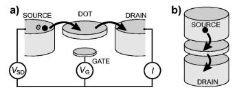
FIG. 1. Schematic picture of a quantum dot in (a) a lateral geometry and (b) in a vertical geometry. The quantum dot (represented by a disk) is connected to source and drain reservoirs via tunnel barriers, allowing the current through the device I to be measured in response to a bias voltage  $V_{SD}$  and a gate voltage  $V_{G}$ .
