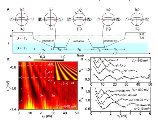
FIG. 48. (Color online) Coherent two-electron spin state rotations. (a) Pulse sequence. (b) Singlet state probability  $P_S$  measured as a function of the pulse time  $\tau_E$  and detuning  $\varepsilon$ . (c) Horizontal cuts through the data in (b) show clear oscillations in  $P_S$ . (d) By increasing the tunnel coupling, a fast  $\sqrt{\text{SWAP}}$  operation time of  $\sim 180$  ps is achieved. Data reproduced from Petta, Johnson, Taylor, et al., 2005.
