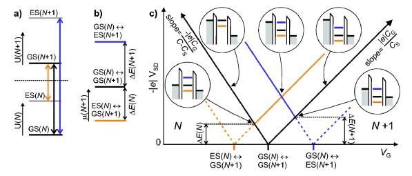
FIG. 5. (Color online) Schematic of a high-bias measurement. (a) Energies for N electrons U(N) and for N+1 electrons U(N+1). Possible transitions are indicated by arrows. (b) The electrochemical potential ladder for the transitions depicted in (a). (c) Schematic plot of the differential conductance  $dI_{DOT}/dV_{SD}$  as a function of  $-|e|V_{SD}$  and  $V_G$ . At several positions the level alignment is indicated with schematic diagrams.
