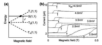
FIG. 37. Dependence of leakage current on the Zeeman energy. (a) Effect of the Zeeman energy on S(1,1) and T(1,1) states, which are separated by an energy J. The S(1,1) and  $T_{-}(1,1)$  states become degenerate when the Zeeman energy is equal to J. (b) Magnetic-field dependence of the leakage current measured at various values of source-drain voltages  $V_{SD}$  in the Pauli blockade region. Each curve is offset by 1 pA from the top. Data reproduced from Tarucha *et al.*, 2006.
