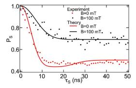
FIG. 47. (Color online) Singlet state probability  $P_S$  measured as a function of separation time  $\tau_S$ . Data points are acquired at B=0 and 100 mT. Solid lines are best fits to the data using a semiclassical model of the hyperfine interaction. Data reproduced from Petta, Johnson, Taylor, et al., 2005.
