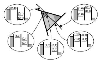
FIG. 31. Level diagrams for different detunings  $\varepsilon$  between dot 1 and dot 2 (dotted line in the bias triangle). Note that the average of the levels in the two dots is kept constant, and only the difference between the levels is changed.
