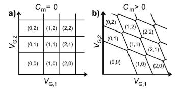
FIG. 27. Charge stability diagrams for (a) uncoupled and (b) coupled double dots, depicting the equilibrium electron numbers  $(N_1, N_2)$  in dots 1 and 2, respectively. The lines indicate the gate voltage values at which the electron number changes. In (b), a finite cross capacitance between gate 1 (2) and dot 2 (1) is taken into account.
