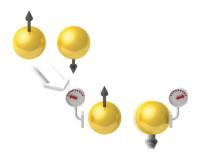
ROTATION: An oscillating magnetic pulse applied to an individual electron can reorient the direction of its spin. The duration of the pulse determines the final direction. The left spin was switched from up to down, and the right spin was put in a superposition state. Rotation is required to load the initial data and perform single-spin operations in quantum algorithms.
