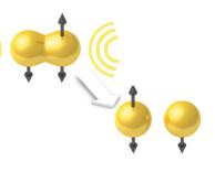
READOUT: After carrying out a quantum algorithm, you need to read out the qubits. Voltage changes to electrodes can push electrons out of their dots. Only the electron with "spin down" makes the jump, because it has a more energetic state. A highly sensitive electrometer detects a current increase, indicating a spin-down electron. No change in current means "spin up." each hold one electron. Electrodes near each dot will control how its electron interacts with its neighbors.
