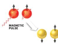
SWAP: Voltage changes to electrodes push the electrons closer together, and their quantum properties become coupled. By being separated after a precise period of time, the two electrons will have swapped their spins. Rotation and swap are basic operations that let you carry out any quantumcomputing algorithm.
